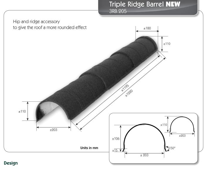
The triple ridge barrel is designed to give your roof a rounded 'finishing' effect. It is pressed from Aluzinc 185 or equivalent metal and available a wide range of colour in granules, satin, brilliance finish to comply with the rest of the roofing materials.
